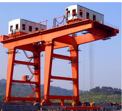
Hydro-power station gantry
