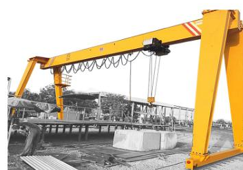
European single girder gantry crane
